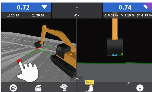
Step 1: Press and hold on plan view to see the "References" menu.
